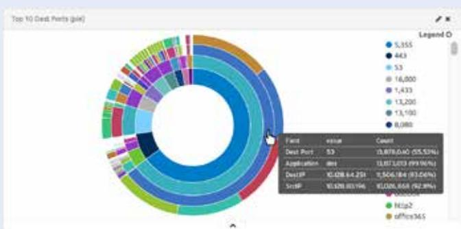
Because of the limited number of DNS query source IP addresses, this indicator is one of the easiest to search for. With a simple filter that looks for DNS traffic without a source IP that matches one of the few servers that host DNS internally, you can quickly find any endpoints that might be compromised.
