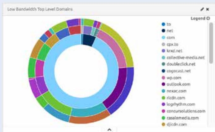
You can configure LogRhythm Network Monitor Freemium's dashboards to show low-bandwidth traffic by top-level domain (shown in this figure as the innermost ring), as well as second-level domains and subdomains (shown as the middle and outer rings, respectively). Metadata, including bandwidth consumption, time of use, and dozens of other pieces of information (on a per-packet or per-flow basis), all provide needed context around the specific nature of suspicious outlier traffic.
